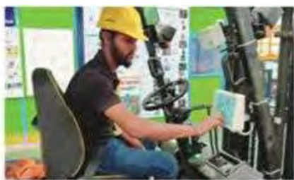
Fixing of load cell sensor & Biometric in Forklift.
