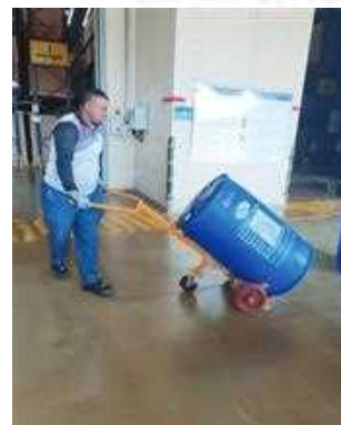
Work place Ergonomics Improvement- Ergonomic study based on ISO standard Introduction of Drum Handling Trolley based on Ergonomic study report
