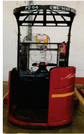
All MHE marking with reflective tape and SWL
