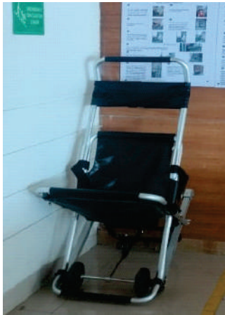
Emergency Evacuation Chair: For safe stairway exit of the disabled, pregnant, or injured.
