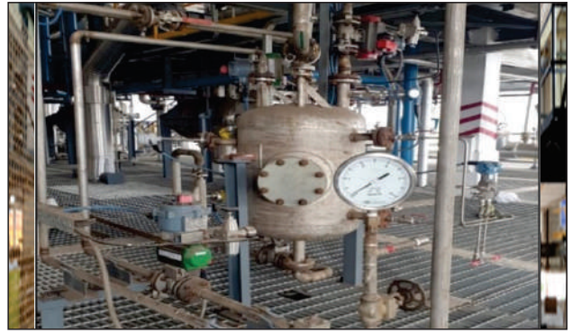
Emergency chain transfer agent auto charging System
