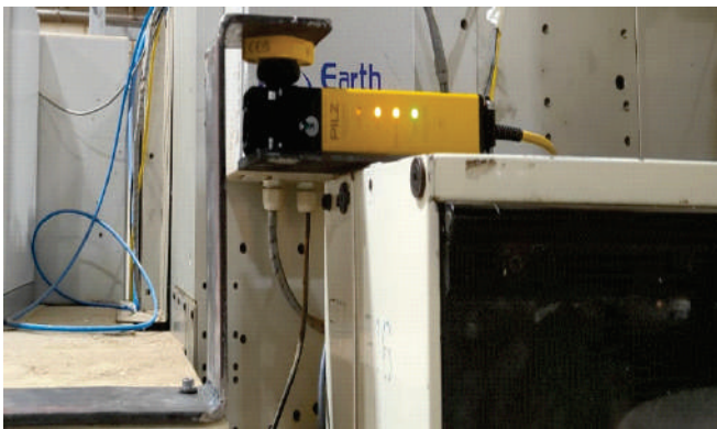
GDX6 : Dead man's Switch | RFID – Coded safety Interlocks prevent override | control supervision are maintained during troubleshooting
