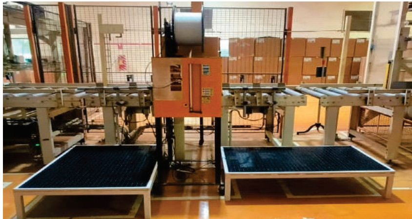
Safety mat for the strapping machine: seamless integration to operations | restrict access during operation
